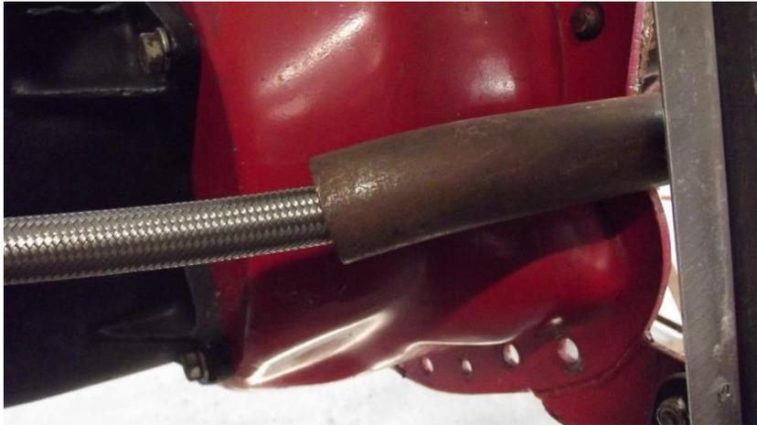
3. S.... A 360-degree driveshaft safety loop is required in the front 25% of the shaft. This needs to be (as a minimum) 1/4" x 1" (6mm x 25mm) steel.
