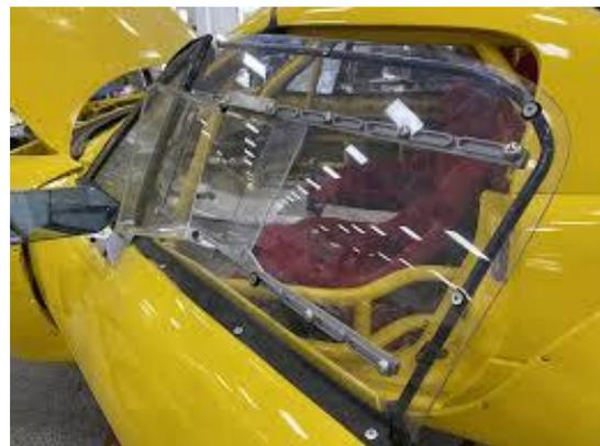
3. U.... If your vehicle has windscreen wipers, they must be removed. If your class record is over 175mph window tabs or straps need to be fitted. (Here are some examples).
