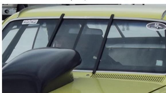
If your vehicle has polycarbonate (Lexan) windscreens, you may be permitted to run without window tabs/straps, provided the windows are mounted SECURELY! (An example in below photo).
