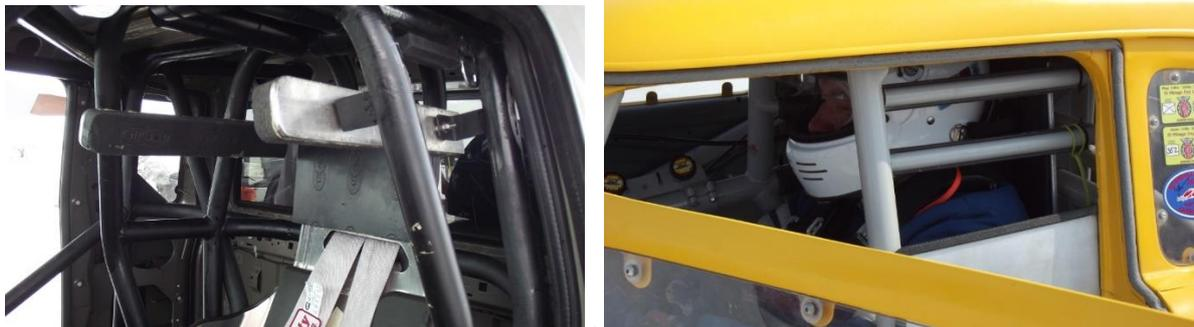
**NOTE:** The restraint must extend to the forward most portion of the helmet as shown above.
