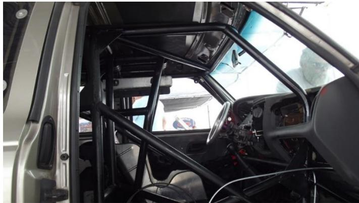
3. B.2.... SFI 45.1(for tube) and SFI 45.2 (for Flat areas) Rollbar padding is required, , the padding must (at a minimum) be placed anywhere the drivers helmet may contact the roll cage, and where ever else you may think necessary.
