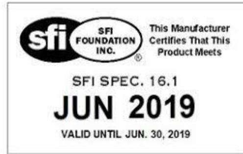
Pictured above right is the new SFI Standard labelling. This label shows that the seat belts were manufactured between 1<sup>st</sup> January 2017, and 30<sup>th</sup> June 2017. Belts now come with either a June or December expiry on them, depending which part of the year they were manufactured. Seat belts with this tag, would be acceptable until June 2022, IF in EXCELLENT condition
