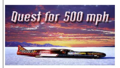
The speed needy brothers formed TEAM Vesco in 1988 and campaigned a variety of power plants before switching to the gas turbine in 1993. In 1999, running the Dempsey World Record Associates-supplied 7-stage Avco Lycoming T55-L-11ASA shaft gas turbine engine mated to the TEAM Vesco custom-built reduction gearbox, the partners reached a top speed of 435.780 m.p.h.
